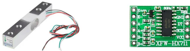
Figure 1. Typical 4-wire load cell (left) and low-cost HX711 PCB assembly (right)
