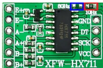
Figure 4. Left: HX711 chip pinout. Right: ADC input channel selection using zero-ohm resistor. Red – selected input is A (default), Blue – selected input is B.
