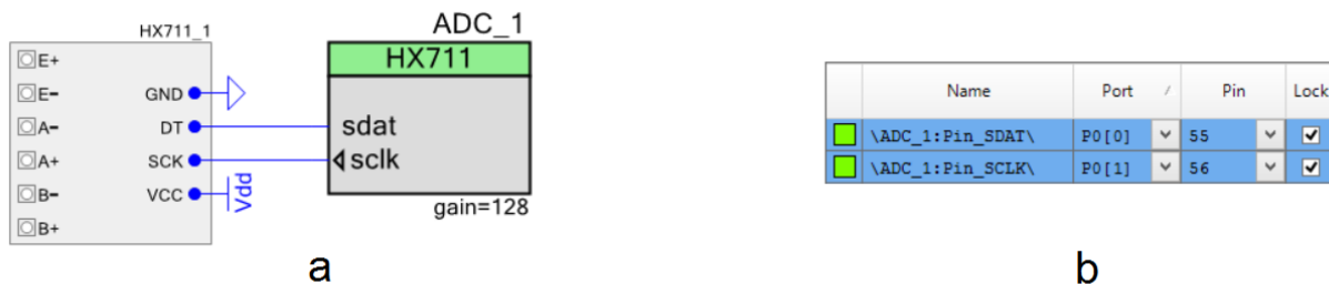
Figure 5. Pins configuration: (a)- component appearance on schematic, (b)- pins assignment. The off-chip annotation component is provided merely for illustration purpose; its presence on the schematic does not affect operation of the component.
