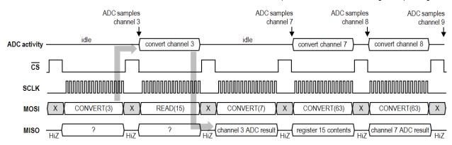
After receiving a CONVERT(C) command, the on-chip ADC samples channel C on the falling edge of the next  $\overline{CS}$  pulse. The analog-to-digital conversion is performed during the next 16 SCLK cycles, and the result is relayed to the master over the MISO line during the following 16 SCLK cycles.
