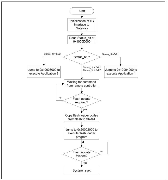
Figure 2 Program flow of bootstrap codes
