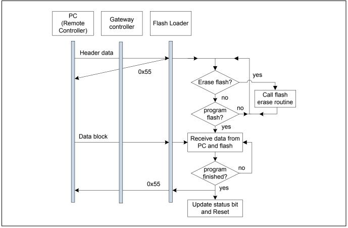
Figure 6 Flash loader procedure for flash programming
