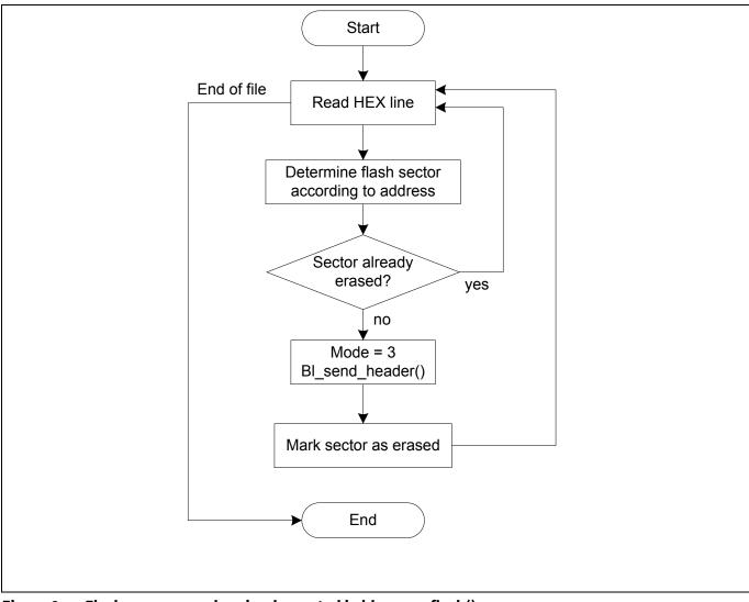
Figure 8 Flash erase procedure implemented in bl\_erase\_flash()
