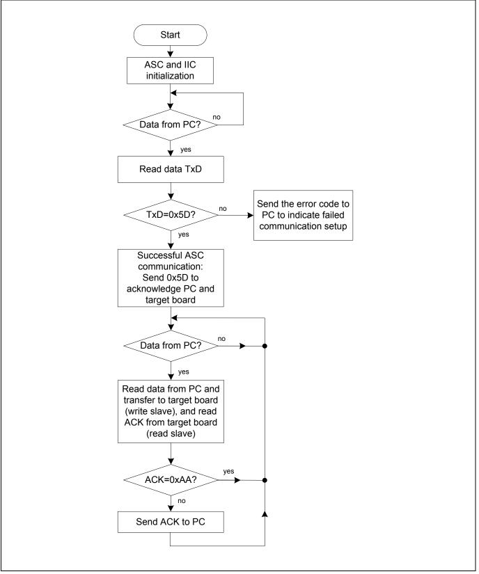
Figure 7 Program flow of the interrupt handler in application codes
