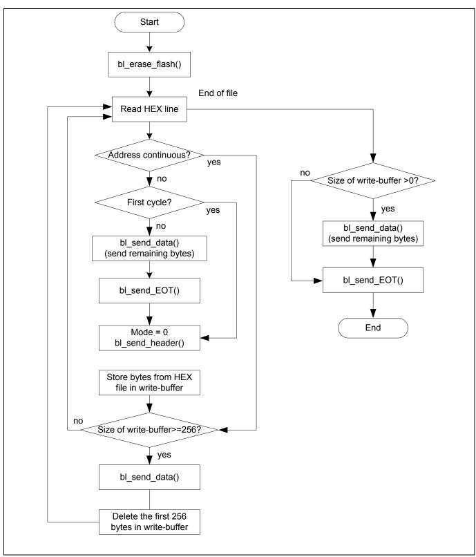
Figure 9 Flash programming procedure implemented in bl\_download\_flash()
