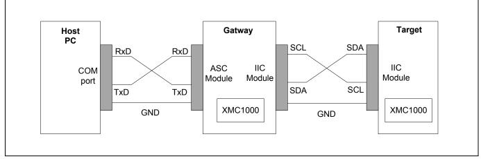
Figure 5 Connection between PC and XMC1000
