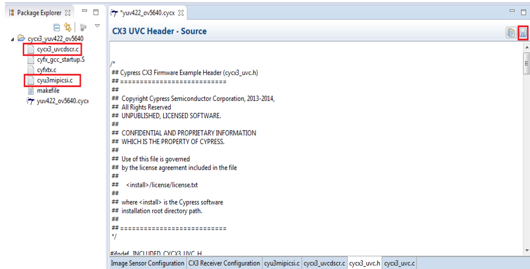
Figure 4-21: Utility generated CX3 Header file
