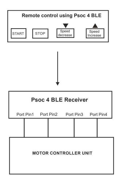
**Motor Control Block Diagram**
