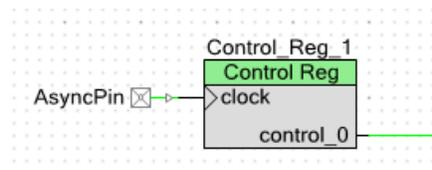
mpr.M0115:Routing of asynchronous signal AsyncPin[0]:iocell.fb as a clock to UDB component "\Control\_Reg\_1:ctrl\_reg\" is not supported unless a UDB Clock/Enable component is used.
