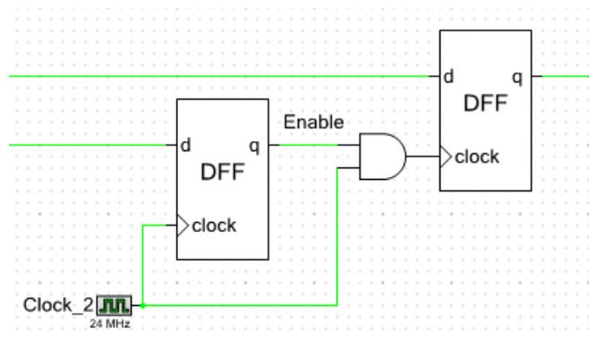
This circuit is implemented with a routed clock, has no timing analysis support, and is prone to the generation of glitches on the clock signal when the clock is enabled and disabled.
