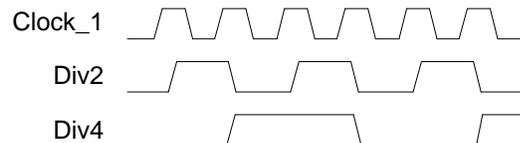
It may appear that the Div4 signal is generated by the falling edge of the Div2 signal. This is not the case. The Div4 signal is generated on the first Clock\_1 rising edge following a rising edge on Div2.
