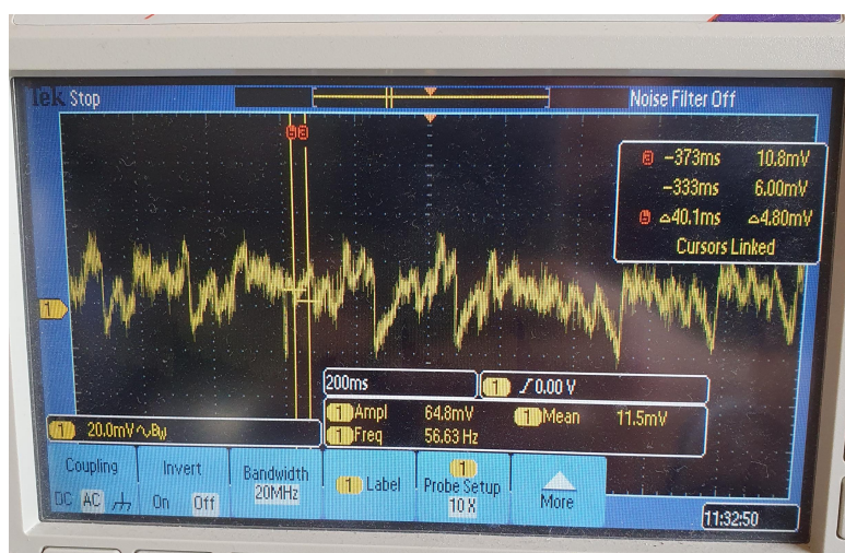
Figure 7.2: Picture of oscilloscope during an AC analysis of the counter electrode vs. analog ground. A 100 nF capacitor is mounted directly to the counter electrode output of the potentiostat.
