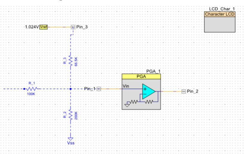
This is my input signal but the voltage peaks is not stable at all..... it can be from 0.3 V to 10V Depending on the intensity of pressure on the sensor.
