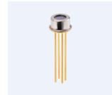
The OTP-638D2 is a thermopile sensor in classic TO-46 housing. The sensor is composed of 116 elements of thermocouple in series on a floating micro-membrane having an active area of diameter 545  $\mu\text{m}$ . The thermopile sensor provides nearly Johnson-noise-limited performance, which can be calculated by its ohmic series resistance. A thermistor with a lead connected to ground is also provided inside the TO package for ambient temperature reference.
