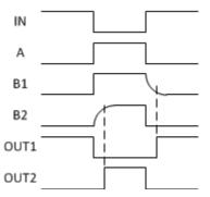
You can see how this circuit reproduces the same non-overlapping outputs that we've seen at the end of
