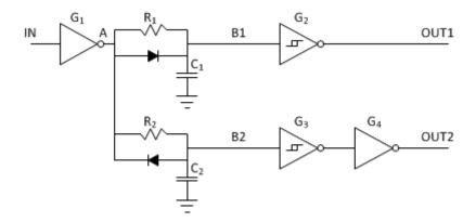
It uses the the R/C circuits to delay the edges of the two outputs, and the diodes to make sure only one of the two edges get delayed. The Schmitt-trigger inverters are needed to clearly define the point where the output switches due to the slow changing of the output of the R/C circuit. The timing diagram of the circuit is the following:
