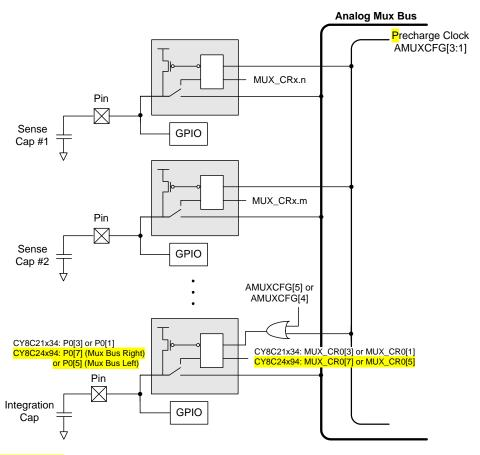
Figure 33-3. CY8C24x94, CY8C21x34, CY8C21x34B, CY7C64215, CY7C603xx, CYWUSB6953 Capacitance Sense Example Diagram
