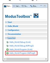
If needed, the IDE builds the application and messages display in the Console. If the build is successful, device programming starts immediately. If there are build errors, then error messages will indicate as such. When complete, the LED will start blinking.
