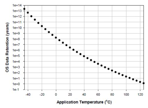
Figure 3. OS Retention Time of Automotive Grade 1 F-RAM at Various Temperatures
