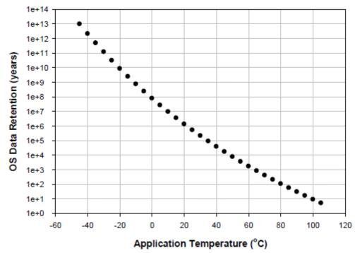
Figure 2. OS Retention Time of Automotive Grade 2 F-RAM at Various Temperatures
