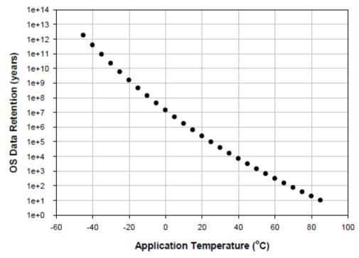
Figure 1. OS Retention Time of Automotive Grade 3 F-RAM at Various Temperatures
