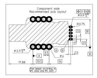
(Layout example with 4 jumpers in parallel)
