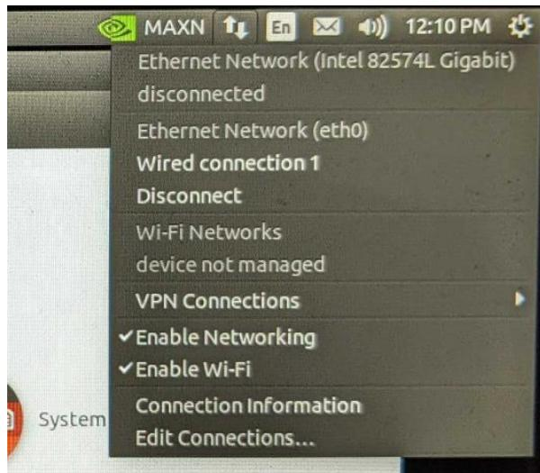
If I edit the "/etc/NetworkManager/NetworkManager.conf" file and comment out the last two lines. I will be able to see and also connect to Wi-Fi access points.
