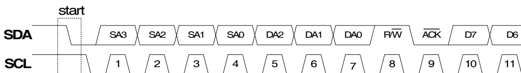
Figure 13-5. Addressing an I2C Peripheral
