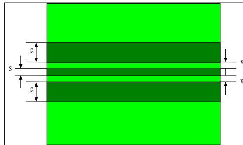
Figure 19. Differential Pairs Placements
