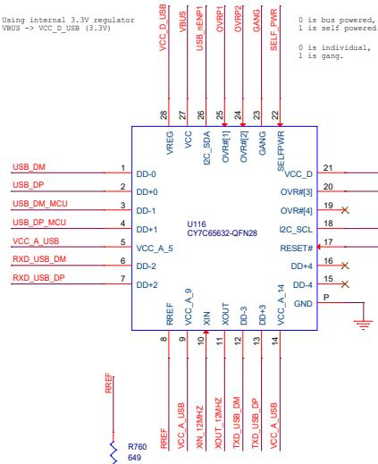
**USB HUB POWERED ON VBUS - it works only when USB cable is connected to USB host**
