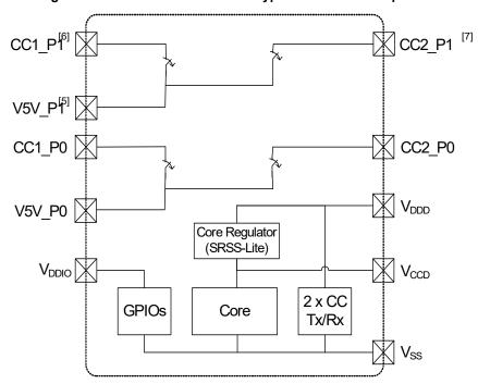
Figure 7. EZ-PD CCG4 Power and Bypass Scheme Example
