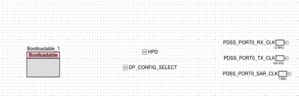
Open TopDesign.cysch file in the PSoC creator project to access dongle’s schematic. Schematic contains hardware resources used by dongle such as clocks, Hot Plug Detect IO etc.
