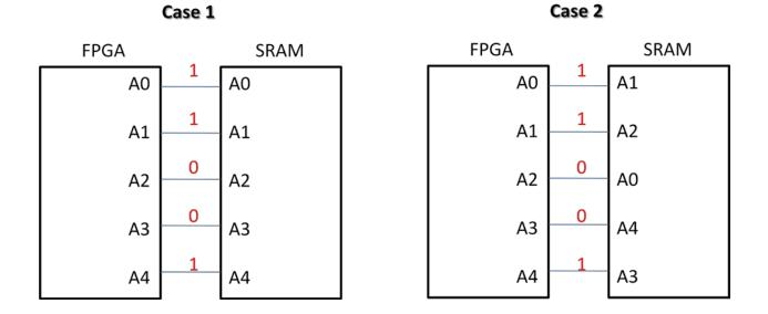
Let's consider an example of Cypress SRAM which has 5 address inputs and interfaced with FPGA. In case 1, if you would like to write a word on address A0, A1, A2, A3, A4 = 11001 then FPGA will send these address bits to SRAM and SRAM will store that word internally on the same address 11001.
