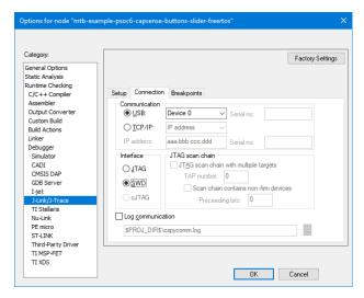
4. Connect a J-Link debug probe to the 10-pin adapter (needs to be soldered on the prototyping kits), and start the debugging session.
