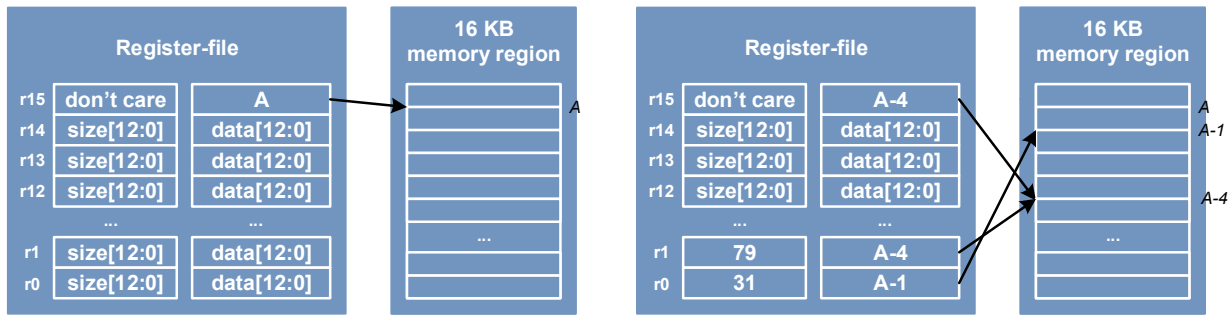
Figure 12-18. Left: Register File State before ALLOC_MEM Instructions; Right: Register File after ALLOC_MEM Instructions
