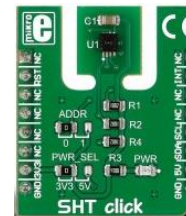
SHT Click Sensor Shield MIKROE-2101
