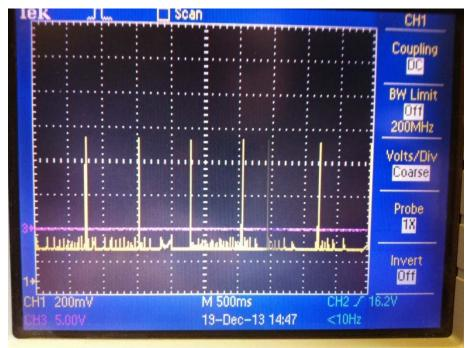
The trace shows the current consumption of the wiced board. The peaks are when the radio exits the very low power sleep mode to receive the beacons and then returns to low power mode.
