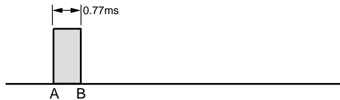
Figure 3. DS18x8 timing diagram with no sensors present. A-Send request, B-data retrieved = empty bus.
