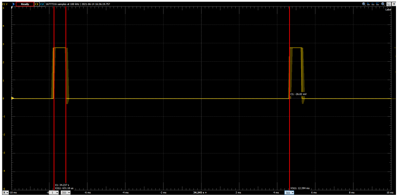
Figure 18 PWM output in train pulse mode (zoomed to pulse)
